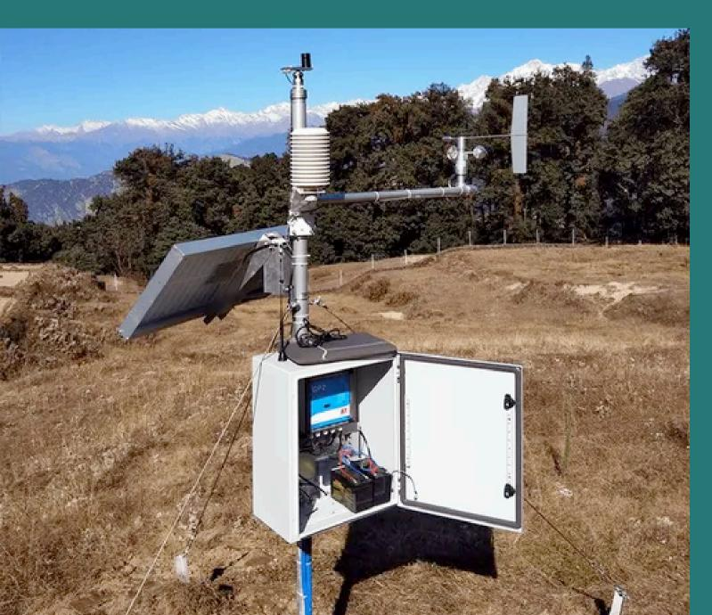
**Sensor Type** Low-cost, solar-powered weather stations **Data Collected** Temperature, humidity, rainfall wind speed & direction **Data Frequency**
