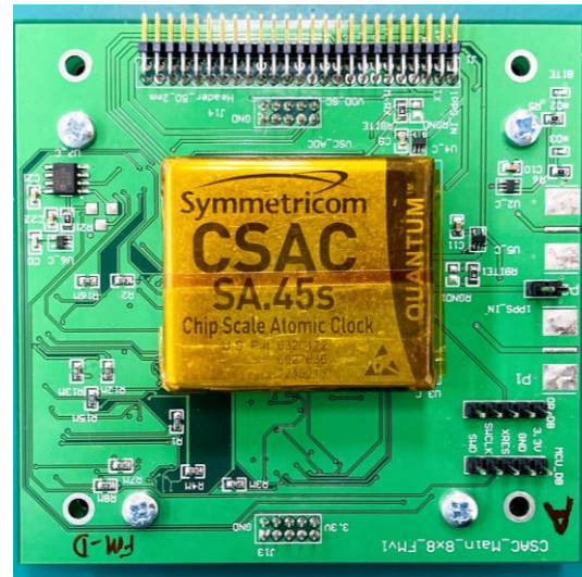
CSAC board designed by NTU (90mm x 86mm)
