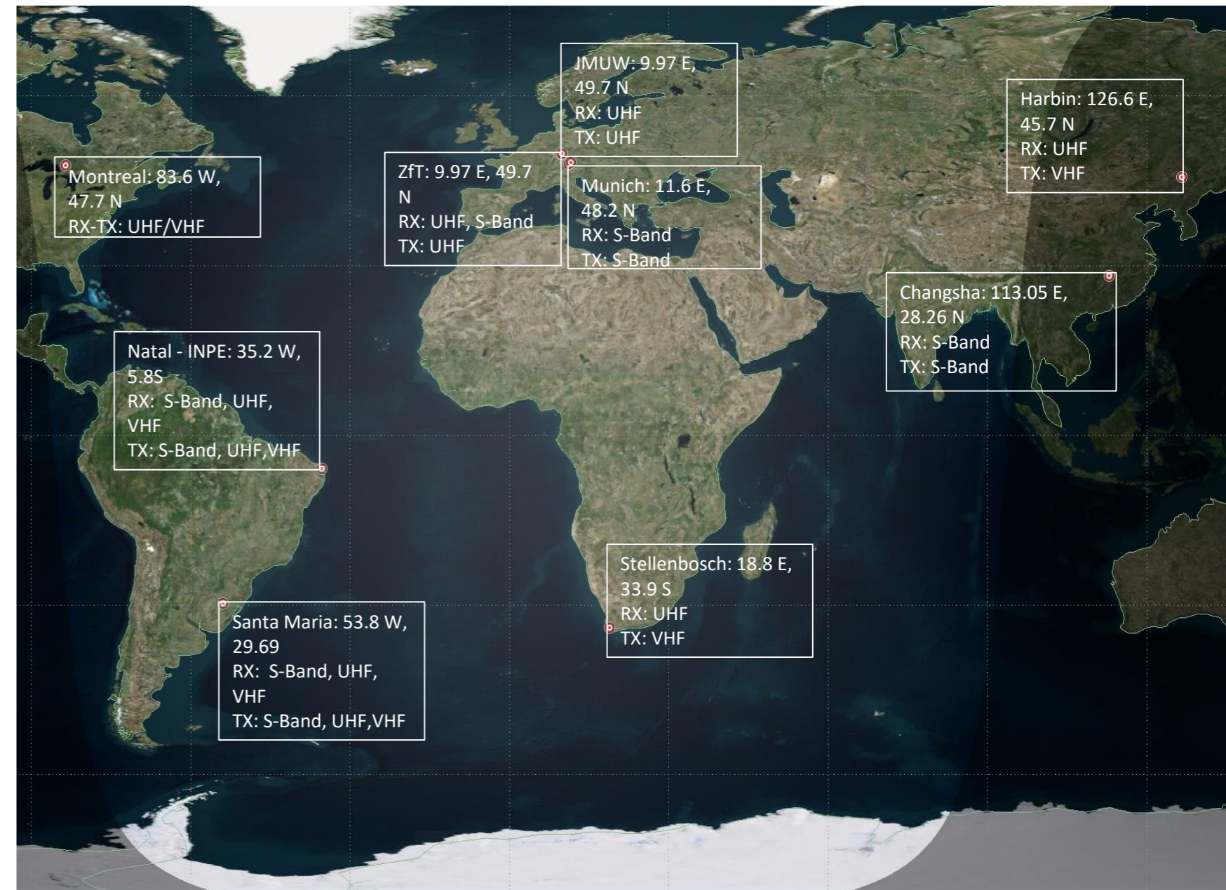
Location and frequency bands of ground stations in TIMGSN
