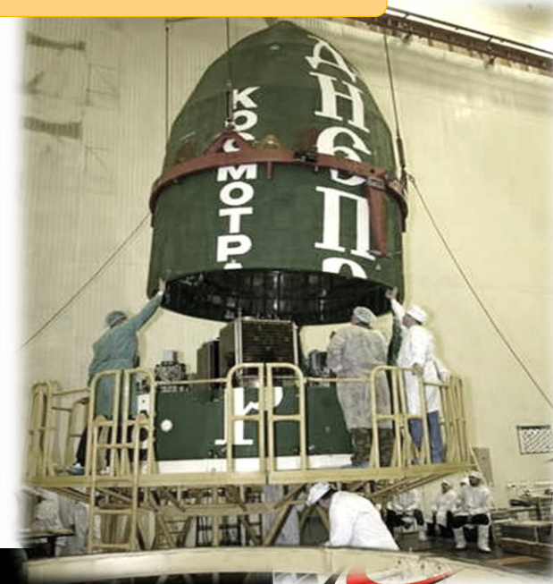
Final Preparation and Installation of EgyptSat-1 to the Launcher
