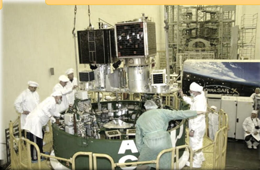
Final Preparation and Installation of EgyptSat-1 to the Launcher
