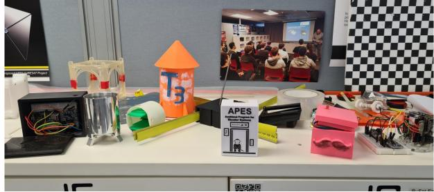
2<sup>nd</sup> Stage: Design P-Sat from scratch using TI MSP processor. Includes circuit design, PCB design & assembly, programming, structure design, communication. Launch to 1km using amateur rocket.
