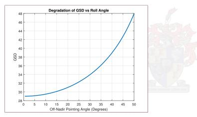
Figure 10: Imager GSD vs Roll Angle
