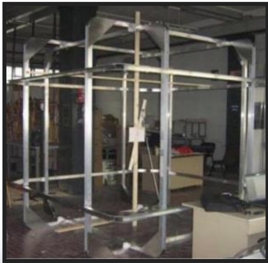
3D Helmholtz coil system
