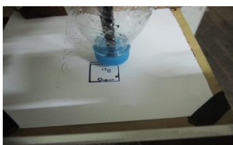
Figure 9: Testing our CNC machine ability of drawing PCB lines
