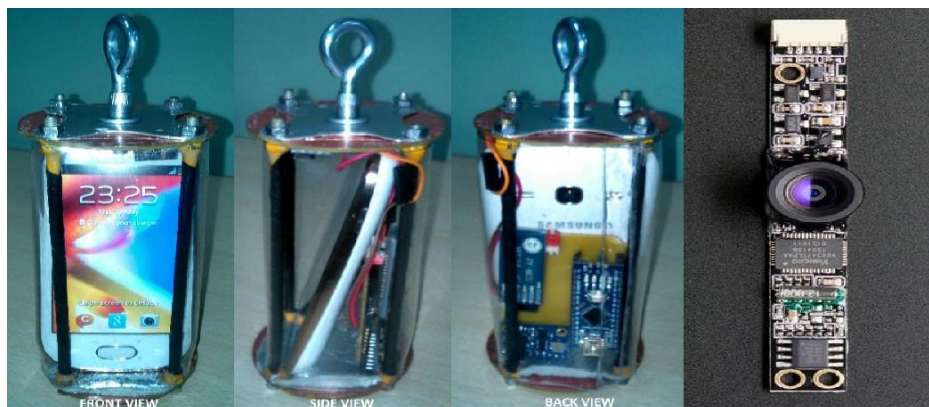
Figure 1: The actual physical framework setup: the Android phone is connected to the Arduino Nano via a Bluetooth module and the Arduino board is connected to a GY-80 Multi sensor board with power and data lines. And “Infragram” USB camera.
