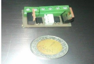
Figure 3: First prototype of motor control module of the rover
