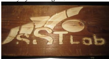
Figure 8: Milling our logo with our shapeoko 2 CNC milling machine
