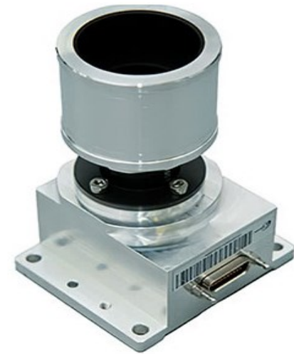
Star Tracker Camera Example - Sodern Auriga
