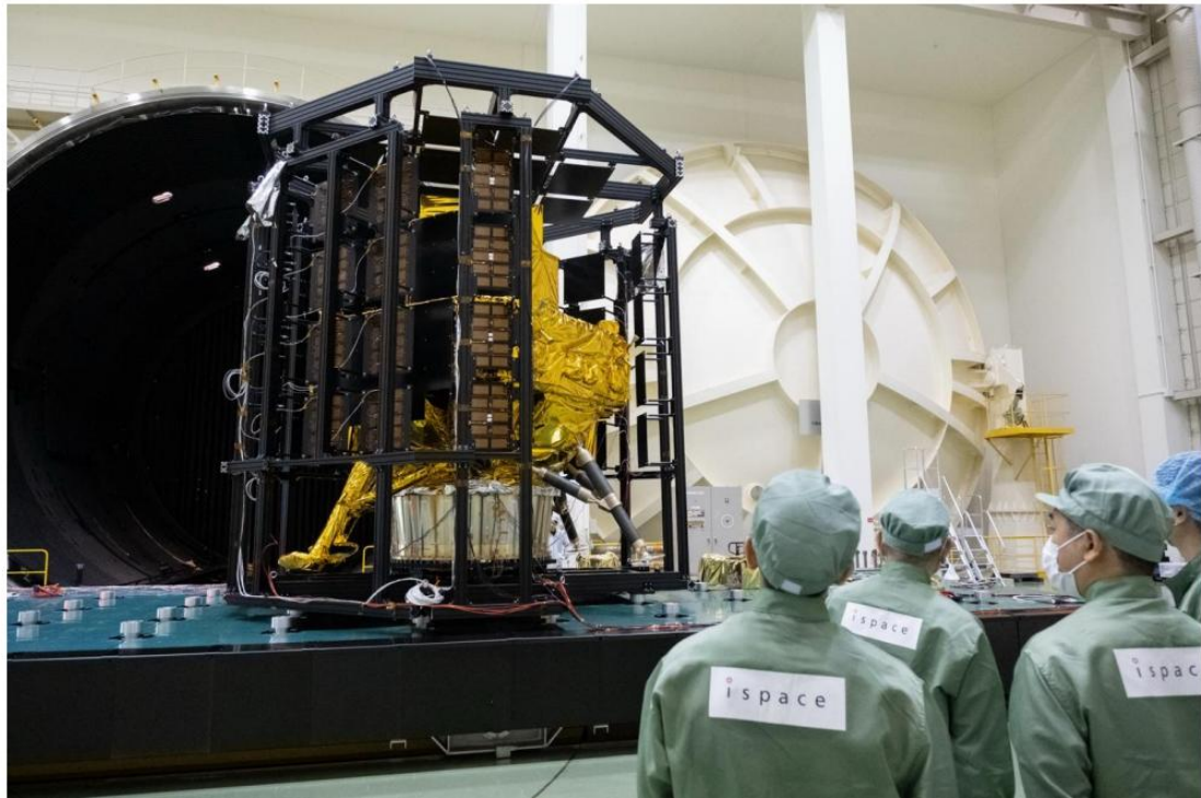
A thermal structure model (STM) of a Series 3 (tentative name) lander is transported from a large thermal vacuum chamber at a JAXA facility in Tsukuba
