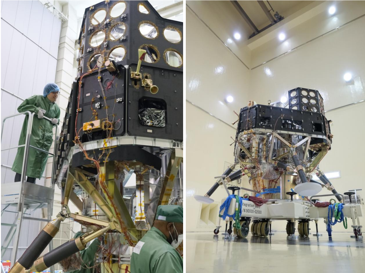
Photos of the structural thermal model of tentatively named Series 3 lander under development with METI's SBIR grant
