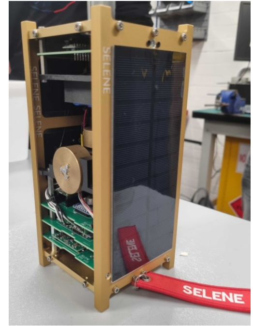
Completed engineering model with side solar panel removed
