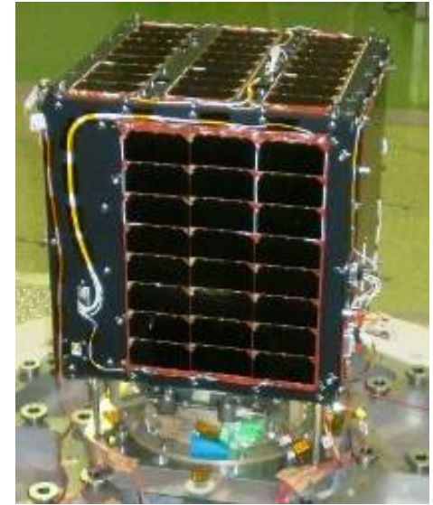
35x35x35cm, 21kg power: 23W C-band downlink only No attitude control
