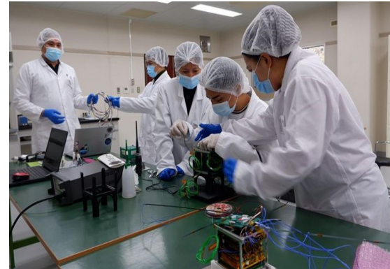
Maya-3 & -4 flight models AIT done by 1st batch of STEP-UP Project scholars (Image credit: DOST)
