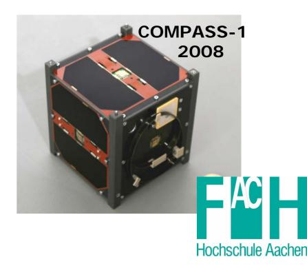
Telecommunication tests: Internet in Space Technology demonstration AOCS: magnetometer, magnetic coils, sun sensors
