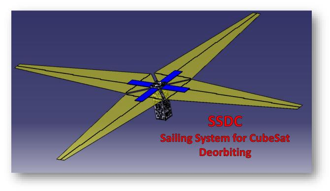
• The designed **SSDC** (**Sailing System for CubeSat Deorbiting**) allows the deorbiting of a CubeSat by exploiting the free and unused volume offered by the standard solar panels without changing the nominal configuration of main subsystems
