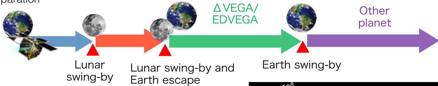
V-infinity leveraging transfer (or  $\Delta VEGA/EDVEGA$ ) can effectively increase the Earth departure  $V_{inf}$ .
