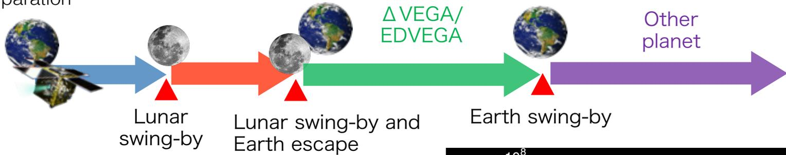
V-infinity leveraging transfer (or  $\Delta V_{\text{VEGA/EDVEGA}}$ ) can effectively increase the Earth departure  $V_{\text{inf}}$ .
