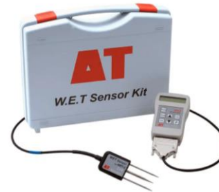
Soil Moisture Sensor (WET-2)
