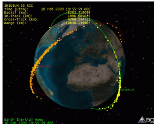
*In 2009, Iridium 33 and Cosmos 2251 collided, originating a debris cloud in LEO. The collision could be avoided by exploiting the satellites Orbit Control sub-system with a collision avoidance maneuver.*
