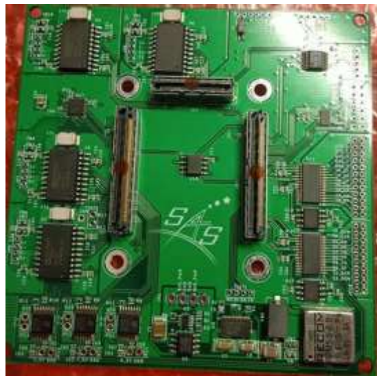
Unit for Telemetry Acquisition and Command Handling (UTACH) Board
