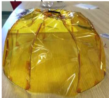
Figure 2: The completed Kapton sail constructed out of eight gores.
