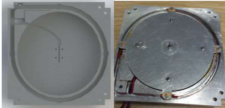
Figure 4 (Above right): A view of the cover lid, secured in place on the sail housing by a Nylon cable, that runs over the four projecting tabs on the lid. A burn wire is routed in the circular channel in the sail housing. The burn wire is set to have four burn locations corresponding to the four points at which the Nylon cable holds down the lid.
